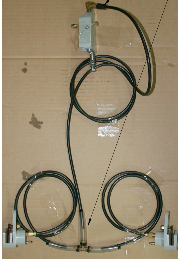
PHOTO SHOWS BRAKE LINE ASSEMBLY (PLUS OTHER PARTS TO SHOW ASSEMBLY CONTEXT)
